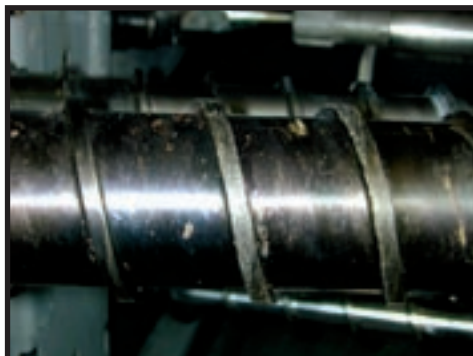
Example of a Screw with Adhesive Wear
