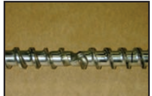
Example of a Screw with Abrasive Wear
